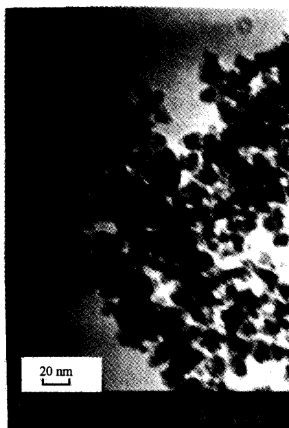
Fig. 2 TEM photo of synthesized Fe 3 O 4 particles.
